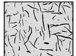
Graphite flakes in the microstructure of the XG-150 cast iron
