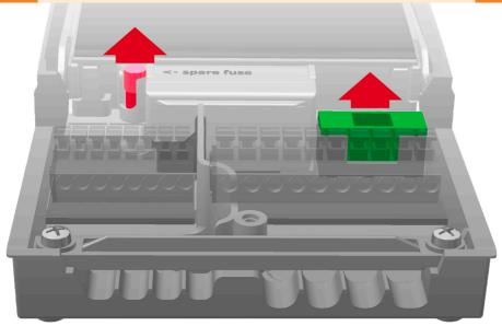
To remove the device fuse, open the terminal cover.
