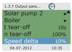
>t tear-off< and >n tear-off< define how long and at which speed the pumps are to run on starting.
