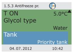
In the case of plants with two tanks, the source of the anti-freeze protection heat must be selected by specifying >Priority tank< or >Secondary tank<.
