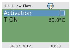
Here, the switch-ON temperature can be defined for low-flow plants.
