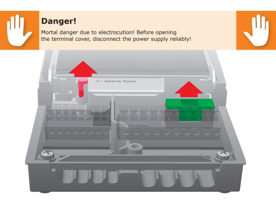
To remove the device fuse, open the terminal cover.
