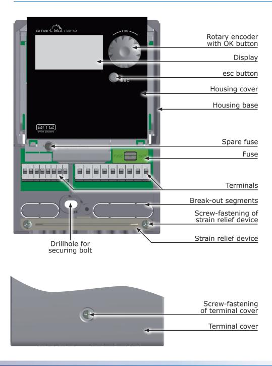
The entire set-up and operation of the differential temperature controller **smart Sol nano** is effected via only two control elements on the device front.
